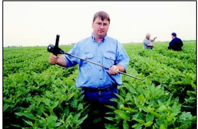
NSW Agronomist Robert Drewitt testing for soil compaction with a penetrometer
